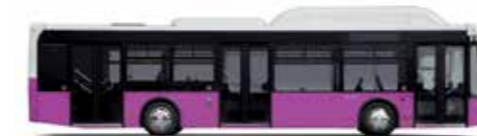
LF 12 CNG L: 12.000 m, H: 3.540 m (with tanks)
